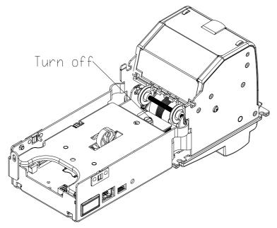
2. When placing cover back, place the right side of the cover first, as shown.
