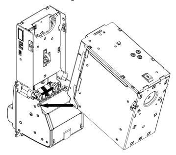
2. Rotate the cassette in the direction of arrow till fasteners of the cassette hook the latches at the validator housing. This action can be done for all types of cassettes whether they are equipped with second metal lock or not, as well as for the "gaming" cassette.
