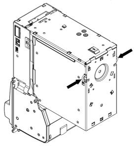
4. To collect bills from the cassette open the lock (or locks) at the cassette cover and open the cover. Remove bills. Close the cover.
