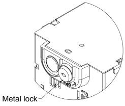
Every cassette can be equipped with the lock that locks the cassette to the bill validator. This optional locking mechanism is placed at the rear side of the cassette and prevents the removal of the cassette from the bill validator.
