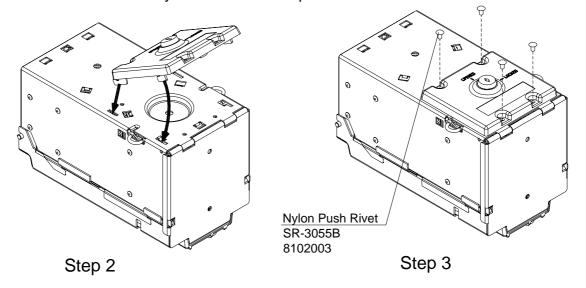
3. Secure the locking mechanism with 4 plastic push rivets.
