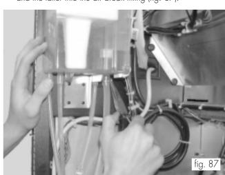
Insert the other spring (ref. I, fig. 79) into the pipe free end (ref. h, fig. 79) and the latter (fig. 88) into the upper fitting of the cartridge support set (ref. a, fig. 79).
