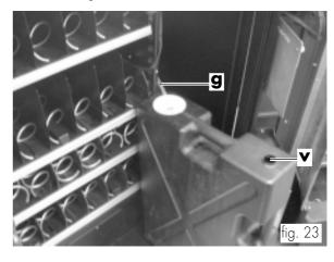
Fit the cap on the tank. Place the tank inside the V.M. (fig. 24) by sliding the pipe inside the tank itself. Close the hole (ref. **v**, fig. 23) by means of the cap (ref. **n**, fig. 9).
