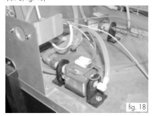
Tighten the relay and support plate (ref. r, fig. 9) by using the screws previously taken from the inlet solenoid valve (fig. 16)
