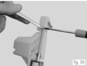
Assemble the whole unit on the sugar stirrer dispenser (fig.
